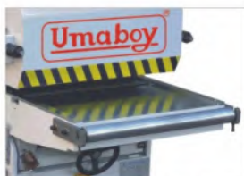
Min. processing length of short material guide is 150mm.
