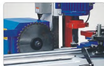
TOP AND BOTTOM CUTTER Tenon cutter for precise tenon with end cutting
