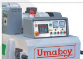
The products is provided with import hd digital display device, which can be operated directly to processing thickness from operating panel with the accuracy up to 0.05mm; be sides, upper and lower planning motor is provided with current meter for visual observing it, is overloaded while working.
