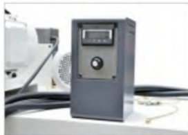
Feeding adopts frequency adjustment, it can adjust the feeding speed according to the hardness of wood.
