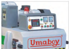
The product is provided with imported digital display device which can be operated directly to processing thickness from operating panel with the accuracy up to 0.05mm blades. upper and lower planning motor is provided with current meter for visual observing if it is overloaded while working.
