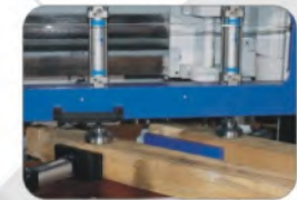
Powerful Pneumatic Clamp For Holding The Frame
