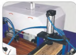
Powerful Pneumatic Clamp For Holding The Frame
